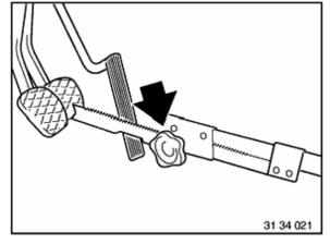
Install pedal support and actuate brake pedal. This prevents brake fluid from escaping from the brake system after the brake line has been disconnected.
