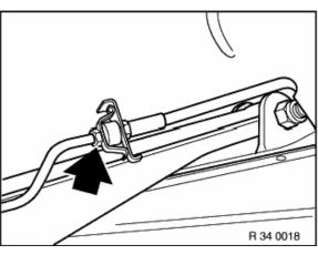
Disconnect left and right brake pipes.
